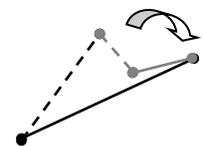
2 – Here we draw 2 separate lines that join at a point however the second line was drawn with the right button.
