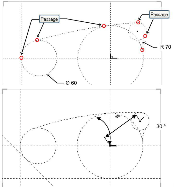
Change the **Line Type** to a thick continuous line. This will be used to trace the required contour.
