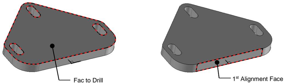
After clicking the first alignment surface, specify a distance of 30mm. The direction of the red arrow indicates the direction of the hole in relation to the alignment surface.
