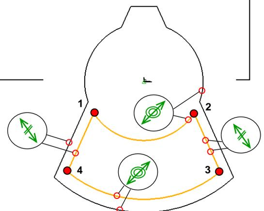
Create the following **Contour** using points. Between the points (1),(2) and the points (3),(4) choose **ARC** **3 POINTS** from the list of options.
