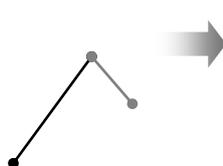
If we move the common point we see that the two lines are in fact separate and can move independently.
