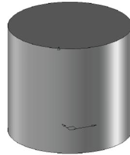
It is possible to combine the coordinate systems with points on coordinate systems with icons showing a red point. For example, in the following case, a coordinate system on face and point will be created, and the point will correspond to a middle point between 2 other points (which are actually the centre points of the 2 circles).
