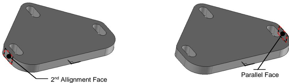
After clicking the 2<sup>nd</sup> alignment face, do not specify a distance; instead click the opposite parallel face. In this case the hole will be constrained at the middle of the two faces.
