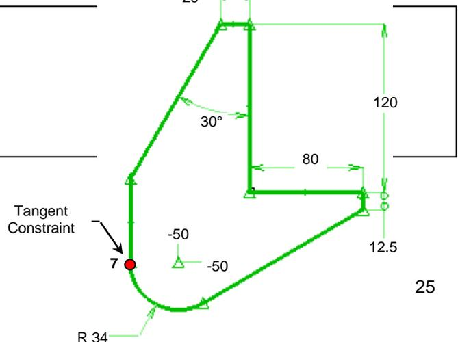
**Dimension** the position of the center of the circle with Cartesian coordinates. Add the dimensions as shown.
