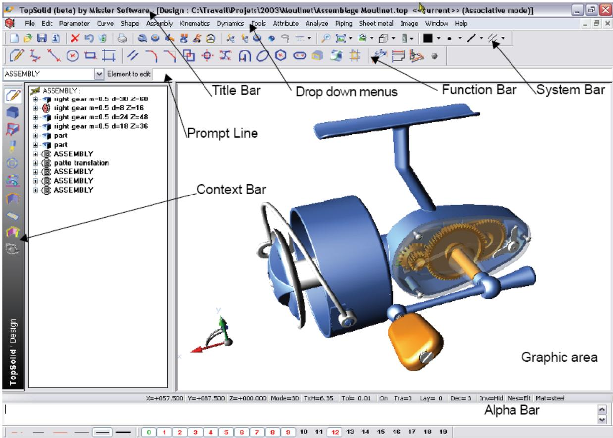
The status bar Provides feedback and allows the user to quickly set layers, colors etc. and set display tolerances and invisible parts. Click directly onto a value to change it.
