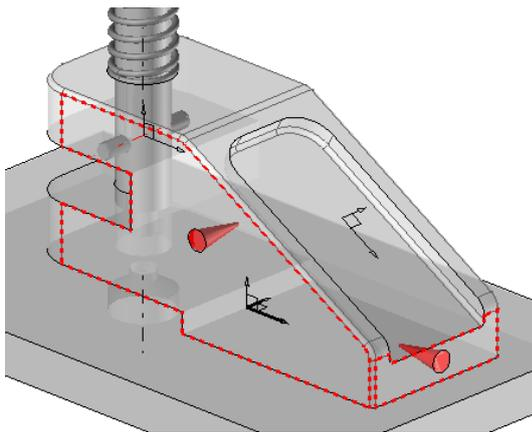
For the parts to fasten, select the Base and Body and then **STOP**
