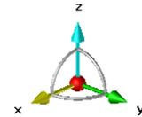
To modify a view, click the **(LM)** of the mouse on a specific part of the compass, then move the mouse keeping the button pressed.
