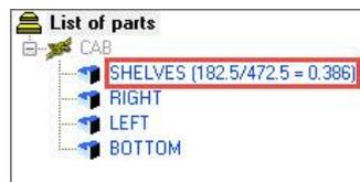
You can configure this ratio in **Tools > Options > Routing configuration > Multi-machining**.
