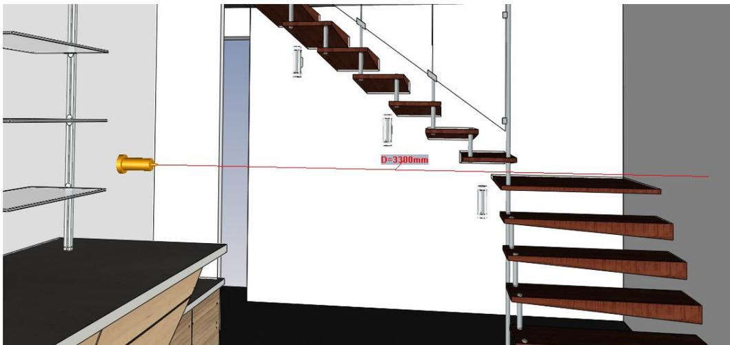
Once the measure is displayed, you can **right-click** on the symbol to bring up a contextual menu that lets you **create the dimension** displayed, **create a distance parameter** that can be reused later, or **create a coordinate system** on the selected face. The **Unhook** option closes the measurement tool.
