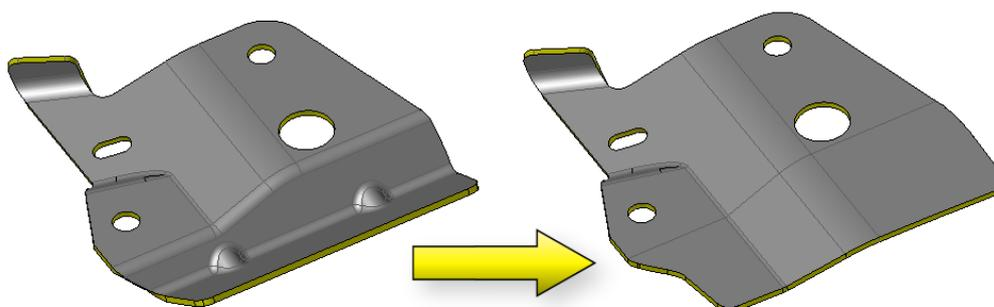
With automatic leading surface mode, the surface that will be used is previewed before the execution of the operation.
