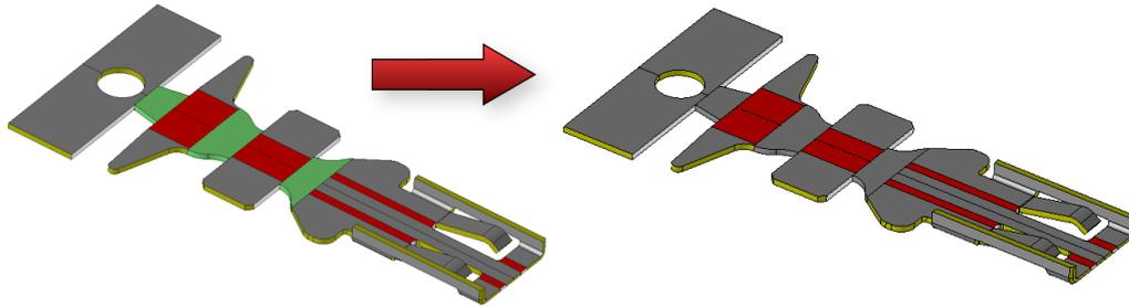
Finally, the **MERGE BODY** function allows you to unite the bodies together before importing the flatten part in order to create the final strip.
