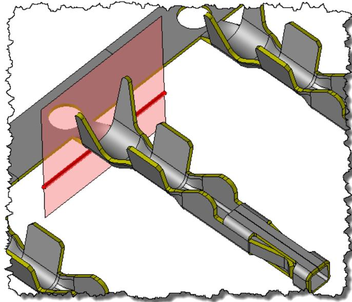
The **REMOVE BODIES** function allows you to remove some of the bodies previously isolated, most of the time, in order to replace it by their equivalent unfolded shapes. The bodies are selected by one of their faces. It is possible to remove several bodies in a row.
