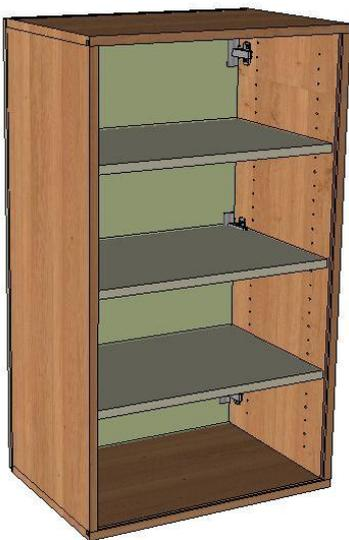
**Example:** A cabinet has a collision between the Hinge pivot and the separation.
