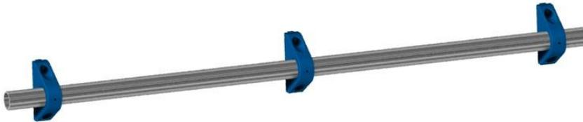
*Example of component, the linear propagation of the blue sub-component has been defined as driver.*
