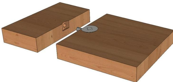
From now, in the assembly template, if a volume (Cylinder or extruded shape) is created in the place where we want create the drilling of the case, only the part that has the collision with the shape will be cut.
