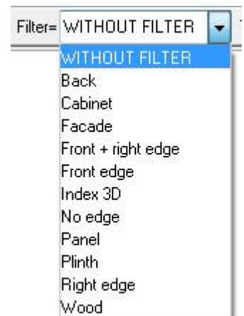
In case this filter chooses the parts according to a property (type, designation...); it is important to apply this property to the **panel entity** and not to the **support**. To do this, launch the **Modify element** function on the panel entity, select **Panel Process**, and then **Modify Cutting-up**. Thereby, the property will be applied to the panel entity.
