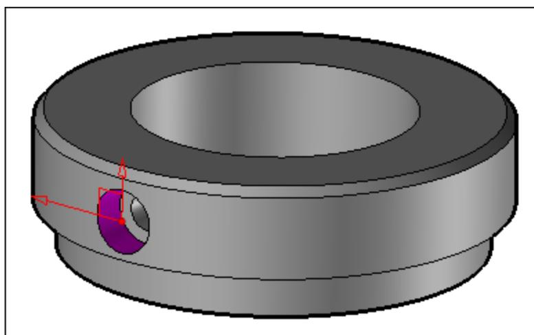
*With imported geometry (basic shape), the reference coordinate of a hole can be quickly created.*
