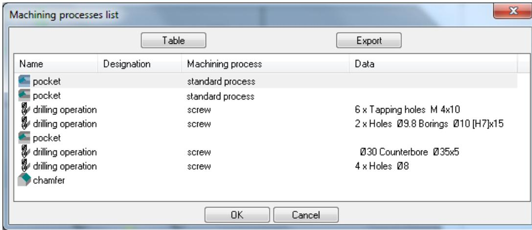
Example of a machining process list for a part.
