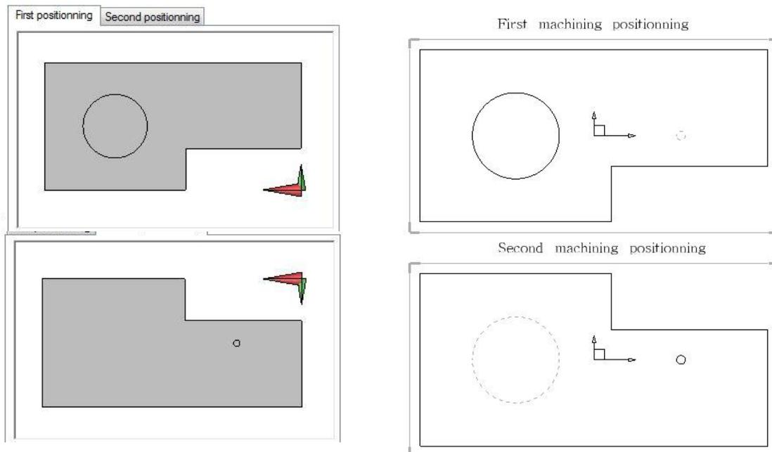
**Scale factor of 2D view:** When positioning the 2D view, we propose you to use the factor 1. In fact, when you use the multiple drafts, the software will calculate automatically the best scale factor to position the view. If the factor is different than 1, it will multiple them with the best factor.
