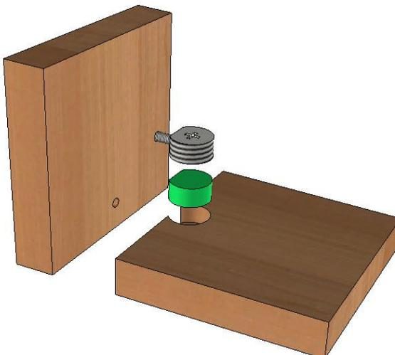
Link the limitation of drilling with the shape
