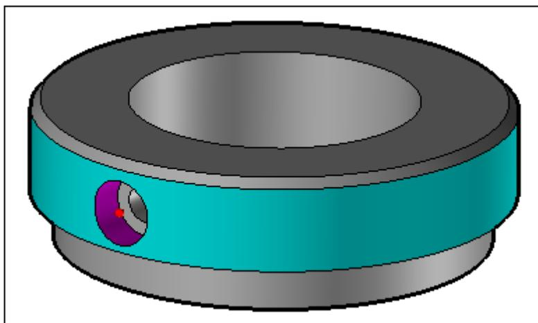
*In magenta: the drilling axis, in blue: the intersected face, in red; the intersection point (reference of the drilling).*
