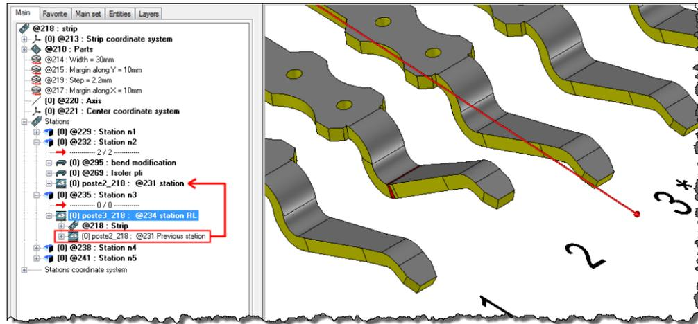
The **Update existing operation to follow** command will redirect the template of the followed operation on the last operation targeted by the insertion operation cursor.
