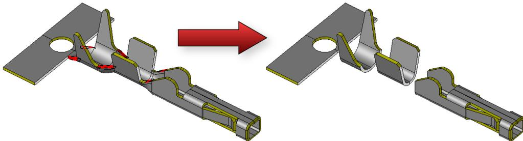
The **MOVE BODIES** function allows you to change the position of some bodies to apply the movement produced by the unfolding of the whole part.
