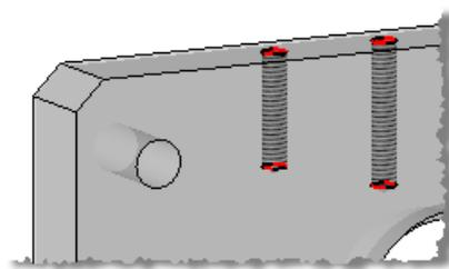
Result of the simplification with merge: the threading face is merged with the hole face.
