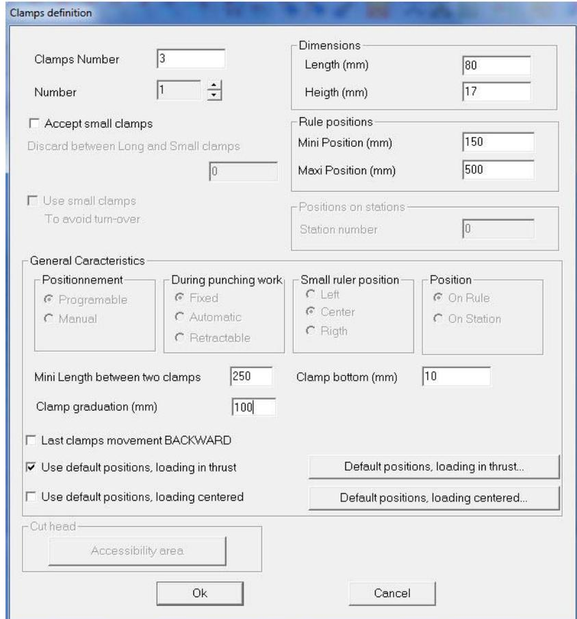
When a non-zero value is indicated, and you have not **used the default clamp positions**, the system calculates the positions by balancing the clamps on the sheet and rounding to the nearest graduation.
