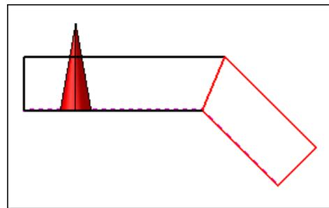
*On the left, the curve to thicken and on the right, the selection of the 1st segment allows you to get 2 thickened curves (in black and red).*
