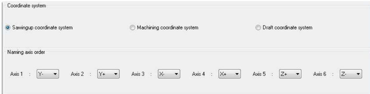
The first edge will be always on the axe 1 refer to the selected coordinate system on the part. (Cutting-up coordinate, machining or Draft).
