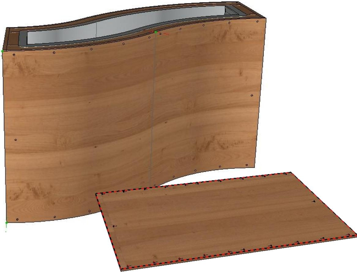
Once the part is unfolded; it is possible, by editing the construction tree to modify several parameters.
