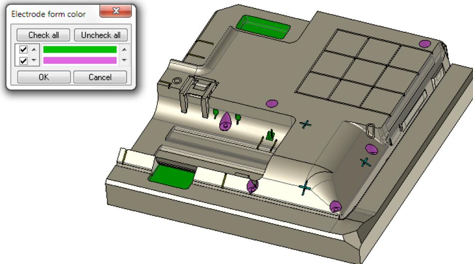
TopSolid'Electrode creates each electrode, as a step by step wizard. Of course, you can manage the parameters for each shape, according to the dimensions of the electrode shell.
