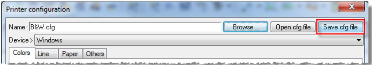
Therefore, several configuration files can be saved according to how the drawings will be printed. Then, when modifying the drawing, the new **Printer** tab allows you to choose the printer, the configuration file, the paper size and the document orientation.
