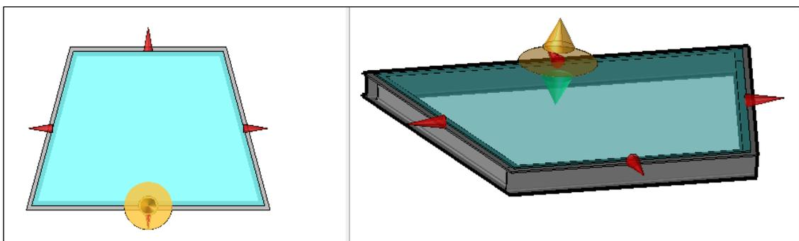
*Example of constrained block creation (in blue) on a trapezoidal structure made up of profiles.*
