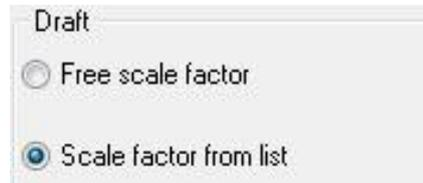
When you use the multi Draft function, the function will automatically calculate the dimension of the 2D view to adapt the dimension of the Draft document:
