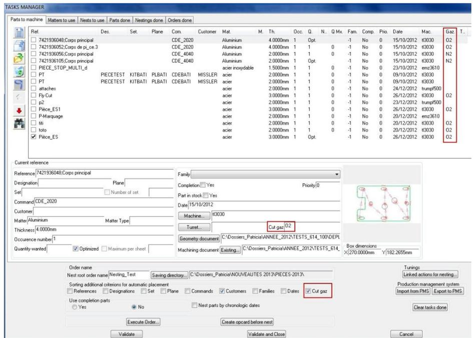
If the additional grouping criterion **Cut Gaz** is not activated, parts with different gases may be mixed.
