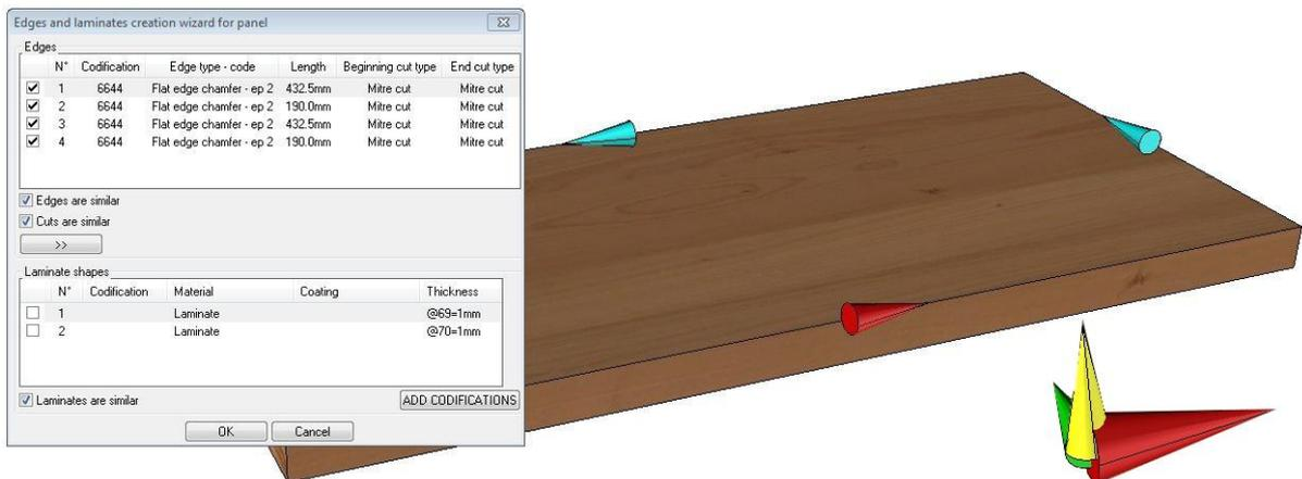
Here the edges are positioned refer to cutting-up coordinate system, 1<sup>st</sup> edge on Y-.
