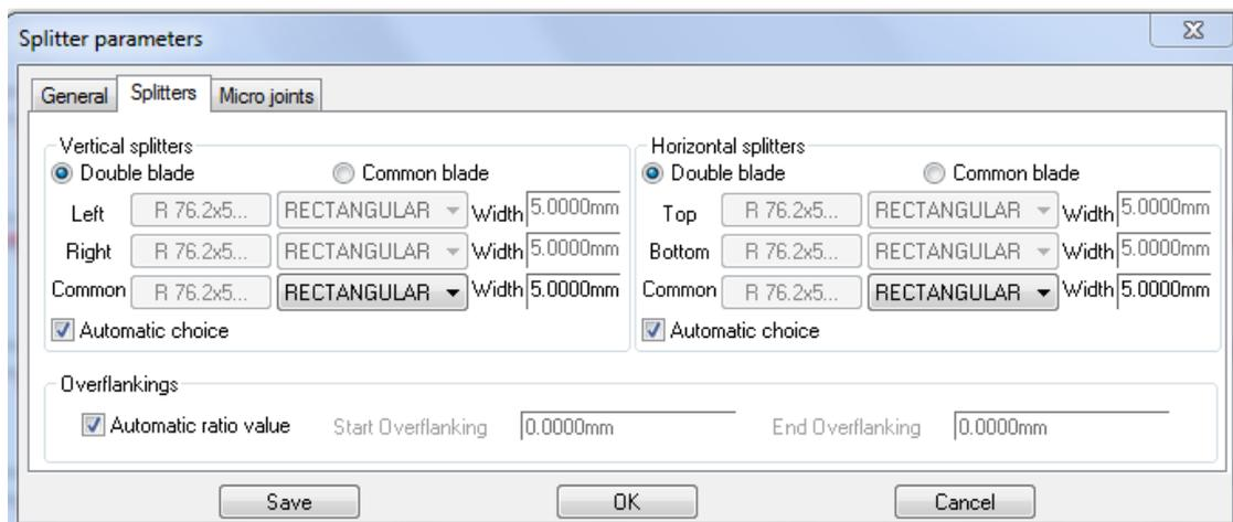
Possibility of using standard functions to locally add, modify and delete micro joints on the splitting lines created. You can also add micro joints manually, or distributed on item. Picking can be carried out on the splitting line created or even directly on the part geometry.
