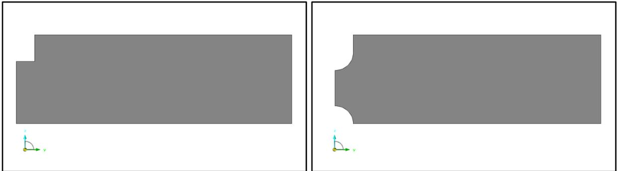
It is now possible to define a CAD operation as a roughing operation. This allows you to indicate to TopSolid'WoodCam to machine this operation, even if no more face of the operation is on the part.
