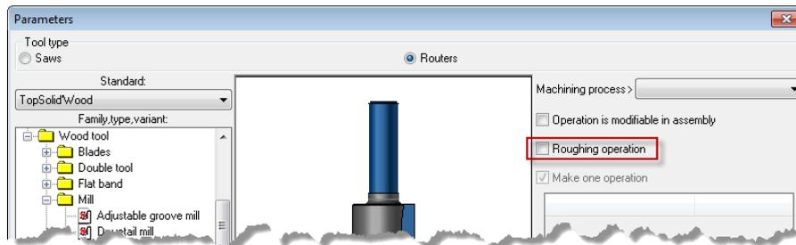
When analyzing operations, if the option is unchecked, the rabbet is not analyzed because it is hidden by the moulding.
