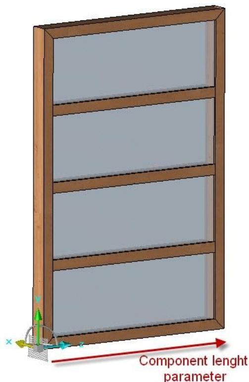
Once you have selected the **DISTRIBUTION** option, you have to select the coordinate system to start it. The selected coordinate system must have the same direction as the component. It means the direction Z+ should be in the direction Z+.
