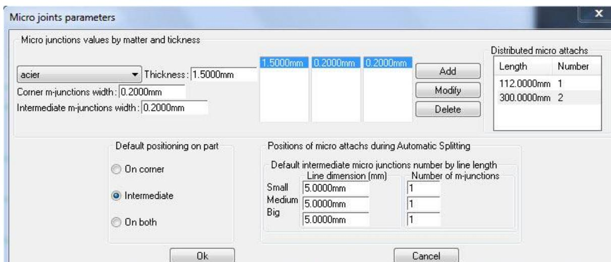
Micro joints are only distributed if the item does not already have micro joints at the start of automatic machining.
