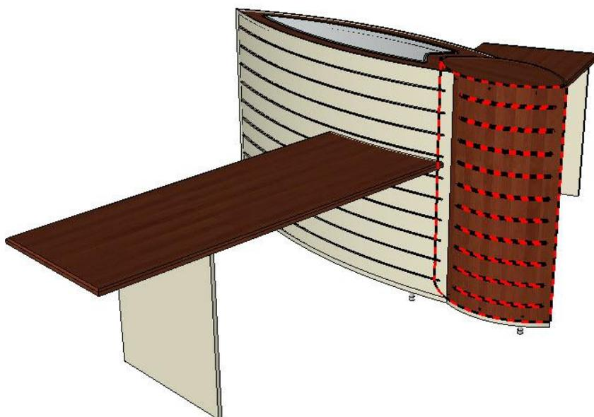
*Unfolded part has the drilling and the start/finish points allow doing the machining on the unfolded part.*
