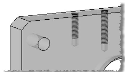
Result of the simplification without merge: the threading faces are identical to the original shape.
