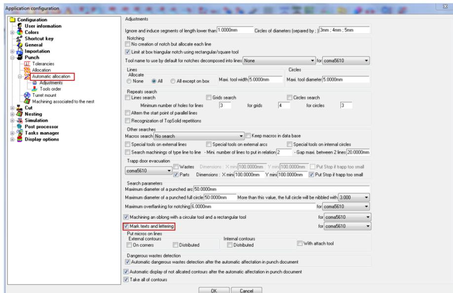
In version V6.14, even if there are two tools with the exact same dimensions: one classified **Normal** and the other classified **Marking**, automatic machining will exclusively select **marking** for lettering, and the **normal** type tool for punched geometries.
