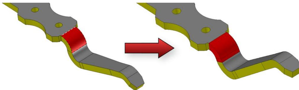
*Reduction of the bend length with a linear additional area.*
