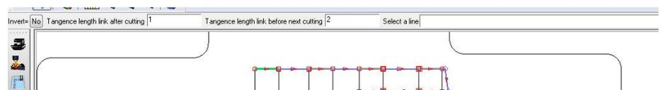
When you have selected a line, it is possible to indicate a tangence length link after cutting and before the next cutting, when there is a change in direction.
