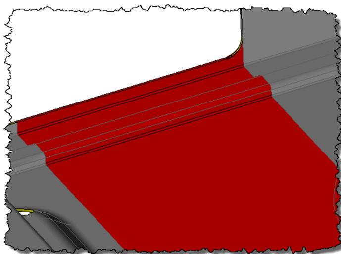
*Result after an unbend for intermediate stage operation.*
