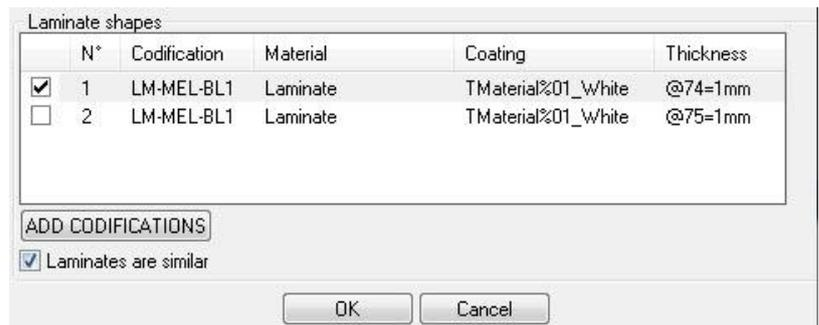
Once you created the laminate codification. It is possible to click on OK to validate the panel configuration window. The codification that you created is added to the TopSolid'Wood library.
