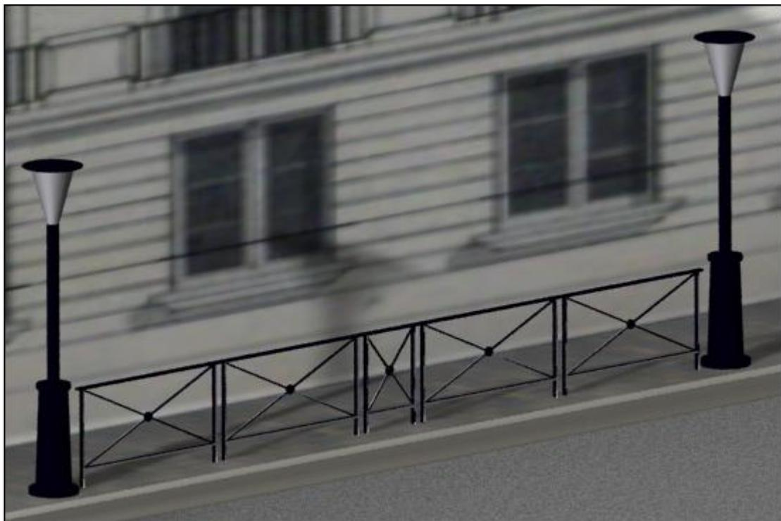
*Example of distribution between two stakes; the midst instance is automatically modified in order to fill the empty space.*
