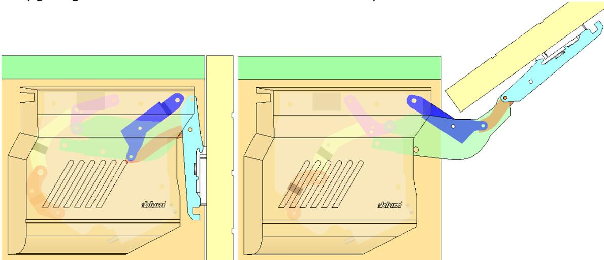
You just need to right-click on the element don't move to make it fixed because the driver block cannot add automatically the constraint. For example as this door, you should right-click on the Hinge pivot and **make it fixed**.
