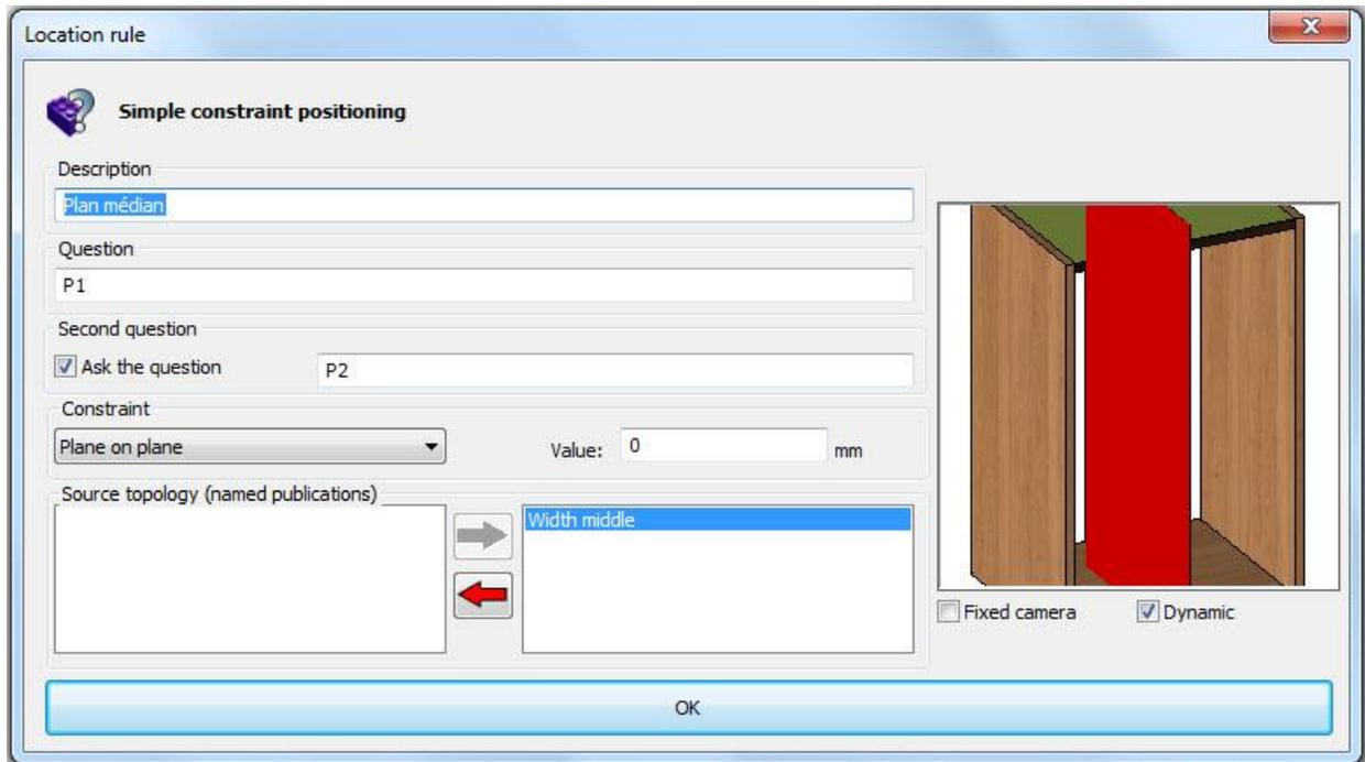
In this example, the **Width middle** publishing will be placed on the plane located between the two faces selected in the questions **P1** and **P2**.
