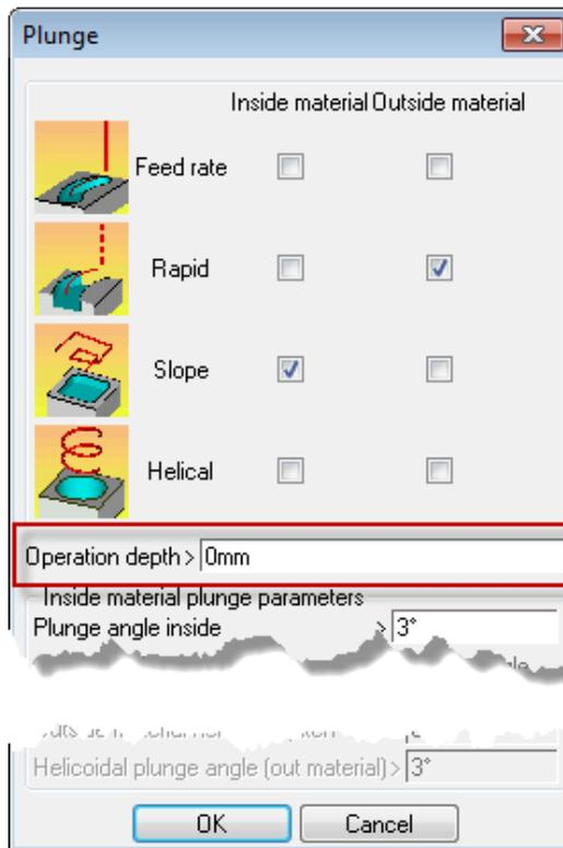
Slope plunge with operation depth at 0mm:
