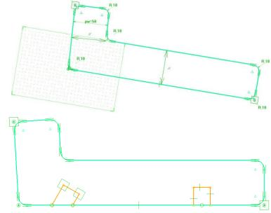
Create two rectangular slots. The back slot is sloped.
